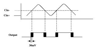
Figure 6-14 Comparator Operating Mode
