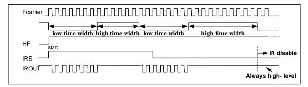
Figure 6-12c LGP=0, HF=1, When IRE goes Low from High, IROUT Pin Outputs Waveform
