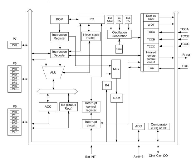
Figure 5 EM78P259N Functional Block Diagram
