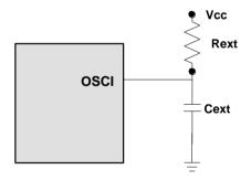
Figure 6-20 External RC Oscillator Mode Circuit
