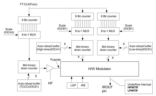
Figure 6-11 IR/PWM System Block Diagram
