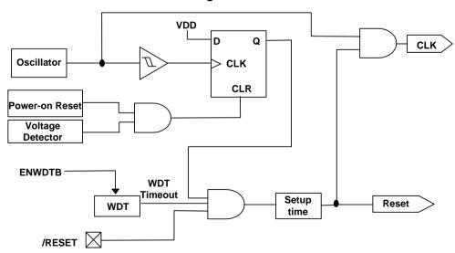
Figure 6-7 Controller Reset Block Diagram
