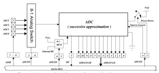
Figure 6-10 Analog-to-Digital Conversion Functional Block Diagram
