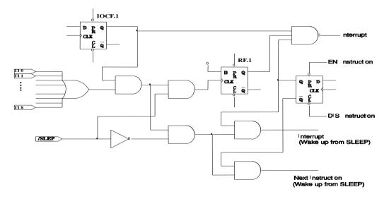
Figure 6-6 Port 5 Block Diagram with Input Change Interrupt/Wake-up
