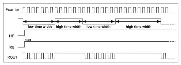
Figure 6-12a LGP=0, HF=1, IROUT Pin Output Waveform
