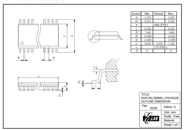
Figure C-7 EM78P259N 20-pin SOP Package Type
