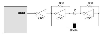
Figure 6-18 Serial Mode Crystal/Resonator Circuit Diagram
