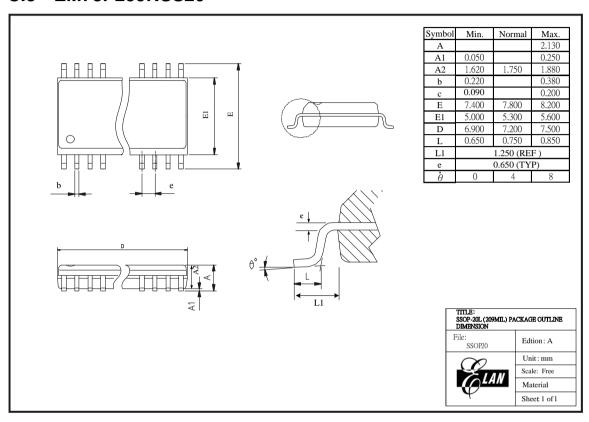
Figure C-8 EM78P259N 20-pin SSOP Package Type
