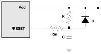
Figure 6-21 External Power-on Reset Circuit
