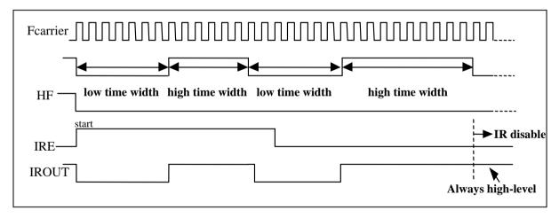
Figure 6-12d LGP=0, HF=0, When IRE goes Low from High, Irout Pin Output Waveform
