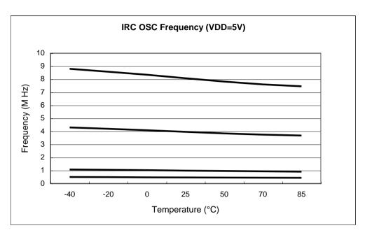
Figure 8-2 Internal RC OSC Frequency vs. Temperature, VDD=5V
