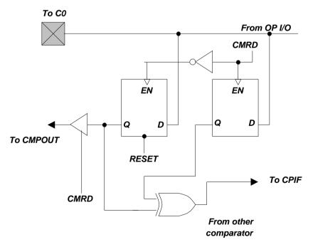
Figure 6-15 Comparator Output Configuration
