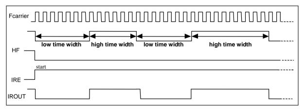
Figure 6-12b LGP=0, HF=0, IROUT Pin Output Waveform
