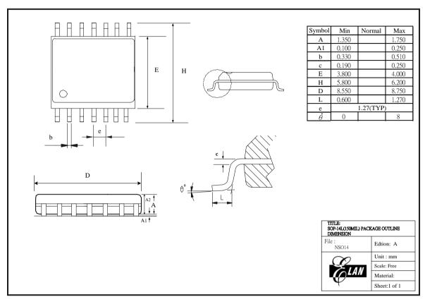
Figure C-2 EM78P259N 14-pin SOP Package Type
