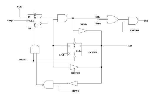
Figure 6-8 Interrupt Input Circuit
