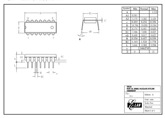
Figure C-1 EM78P259N 14-pin PDIP Package Type
