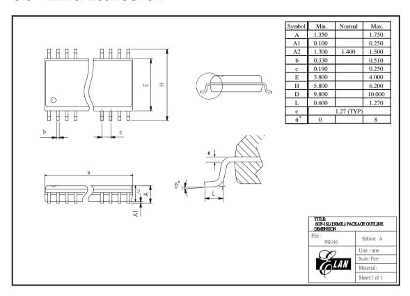
Figure C-3 EM78P259N 16-pin SOP Package Type
