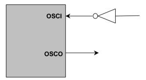
Figure 6-16 External Clock Input Circuit
