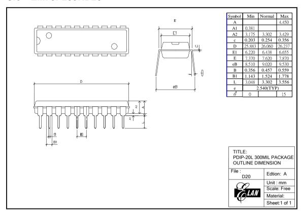
Figure C-6 EM78P259N 20-pin PDIP Package Type
