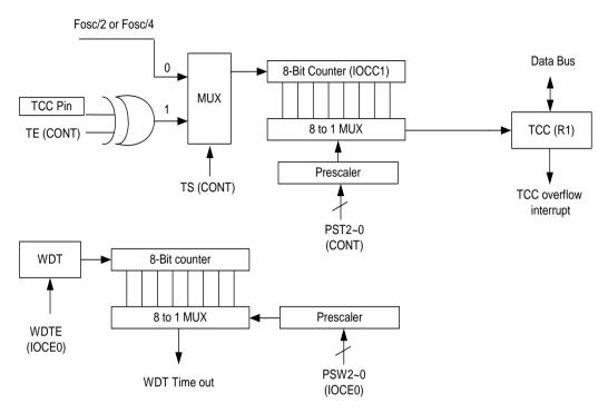
Figure 6-2 TCC and WDT Block Diagram
