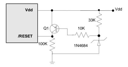
Figure 6-22 Residual Voltage Protection Circuit 1
