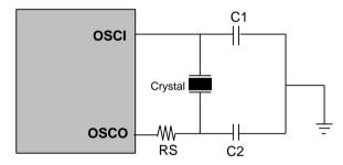
Figure 6-17 Crystal/Resonator Circuit
