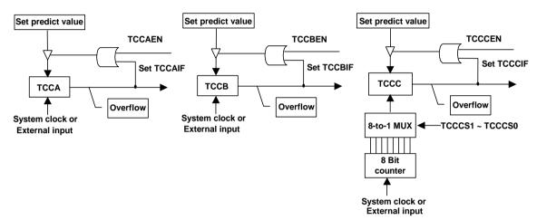
Figure 6-13 Timer Block Diagram
