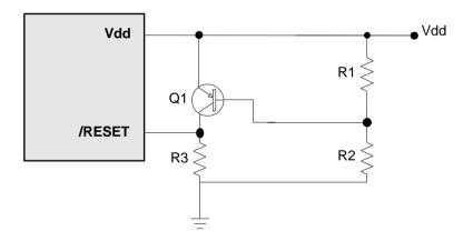
Figure 6-23 Residual Voltage Protection Circuit 2
