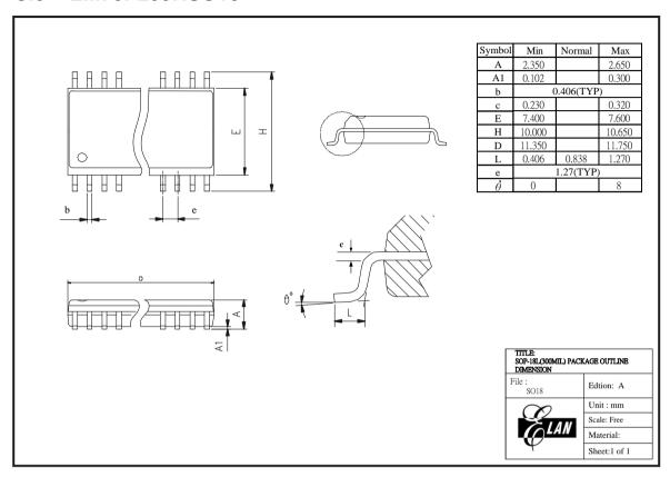
Figure C-5 EM78P259N 18-pin SOP Package Type
