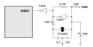
Figure 6-19 Parallel Mode Crystal/Resonator Circuit Diagram
