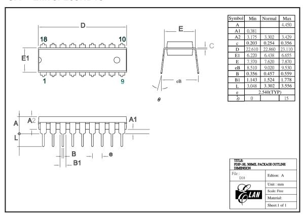
Figure C-4 EM78P259N 18-pin PDIP Package Type
