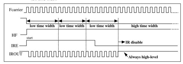
Figure 6-12e LGP=1 and HF=1, IROUT Pin Output Waveform
