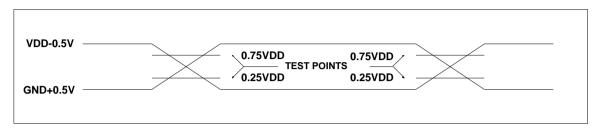
AC Testing: Input is driven at VDD-0.5V for logic "1",and GND+0.5V for logic "0".Timing measurements are made at 0.75VDD for logic "1",and 0.25VDD for logic "0".
